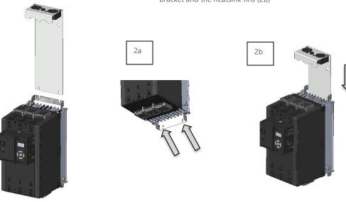
Step 3. When the fan assembly is fully inserted and the lower plate of the assembly has engaged with the lower mounting screws, re-tighten the mounting screws fully.
