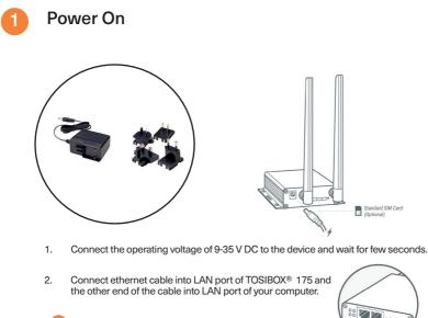
TOSIBOX® 175 LAN port is DHCP enabled. Your computer receives the IP address from TOSIBOX® 175.
