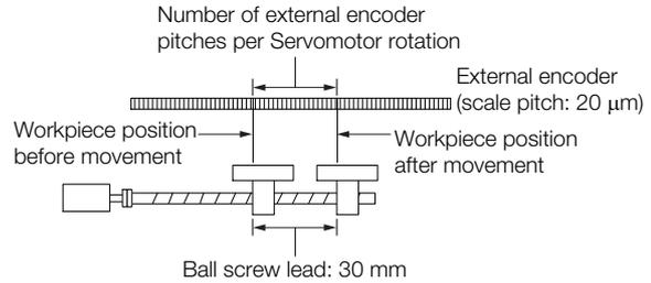
If the external encoder is connected directly to the Servomotor, the setting will be 1,500 ( $30 \text{ mm}/0.02 \text{ mm} = 1,500$ ).
