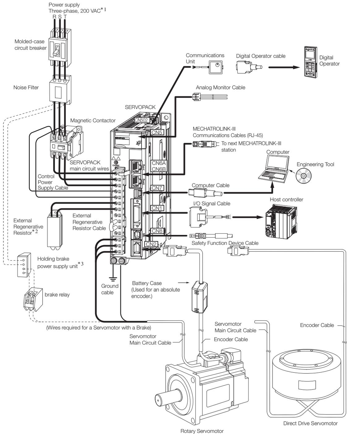
\*1. This example is for a SERVOPACK with a three-phase, 200-VAC power supply input. The pin layout of the main circuit connector depends on the voltage.
