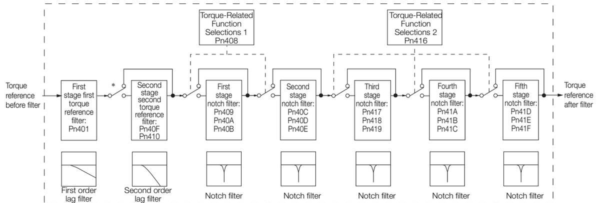
\* The second stage second torque reference filter is disabled when Pn40F is set to 5,000 (default setting) and it is enabled when Pn40F is set to a value lower than 5,000.
