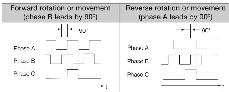
Note: The pulse width of the origin within one encoder rotation depends on the setting of number of encoder output pulses (Pn212) or the encoder output resolution (Pn281). It is the same as the width of phase A. Even for reverse operation (Pn000 = n.□□□1), the output phase form is the same as shown above.
