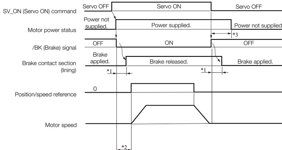
\*1. Rotary Servomotors: The brake delay times for Servomotors with Holding Brakes are given in the following table. The operation delay times in the following table are examples for when the power supply is switched on the DC side. You must evaluate the actual brake delay times on the actual equipment before using the application.
