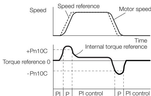
■ Using the Speed Reference as the Mode Switching Condition
