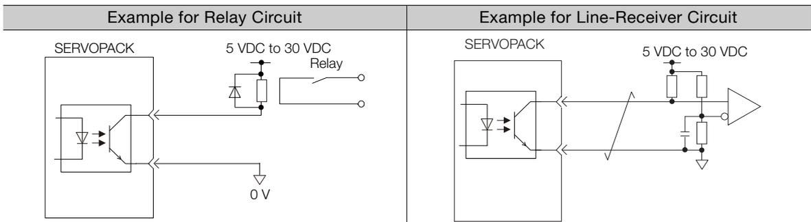
Note: The maximum allowable voltage and current range for photocoupler output circuits are as follows:
