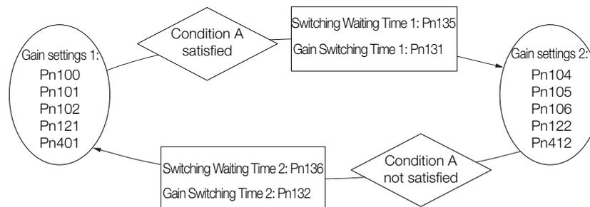
◆ Relationship between the Waiting Times and Switching Times for Gain Switching
