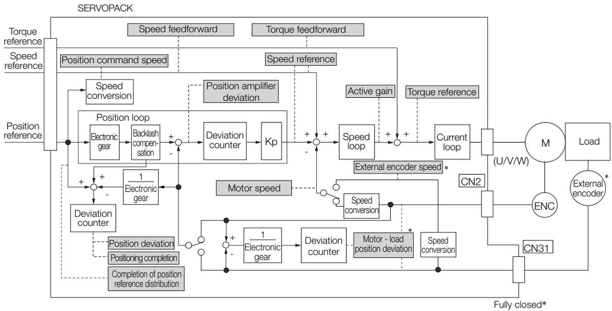
\* This speed is available when fully-closed loop control is being used.
