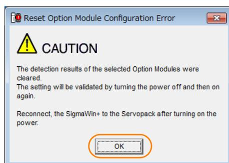
6. Turn the power supply to the SERVOPACK OFF and ON again.
