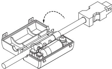
3. Remove the old Battery and mount a new Battery.
