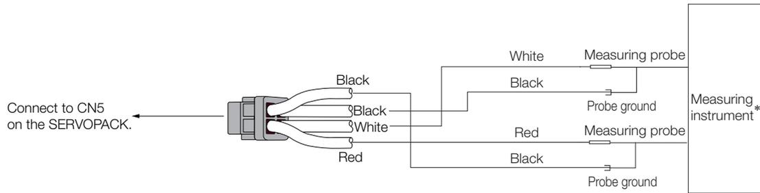
\* The measuring instrument is not provided by Yaskawa.
