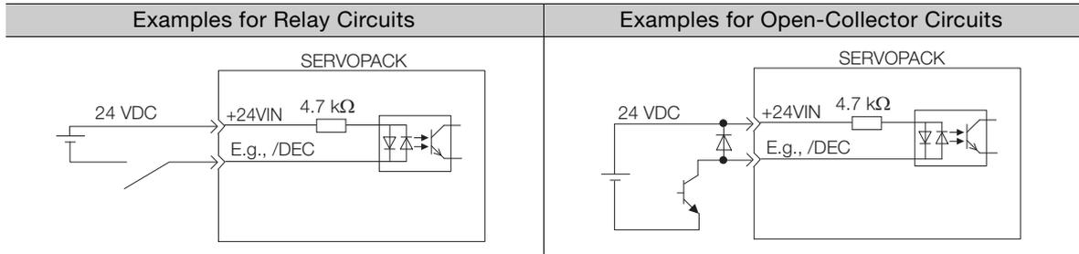
Note: The 24-VDC external power supply capacity must be 50 mA minimum.
