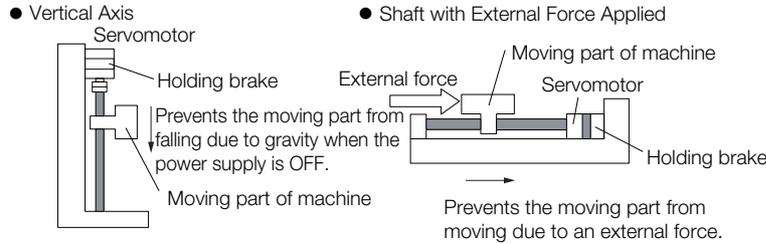
**Important** The brake built into a Servomotor with a Brake is a de-energization brake. It is used only to hold the Servomotor and cannot be used for braking. Use the holding brake only to hold a Servomotor that is already stopped.
