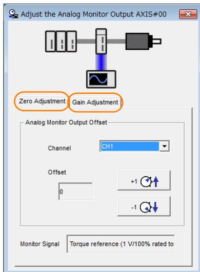
4. While watching the analog monitor, use the **+1** and **-1** Buttons to adjust the offset. There are two channels: CH1 and CH2. If necessary, click the down arrow on the **Channel** Box and select the channel.
