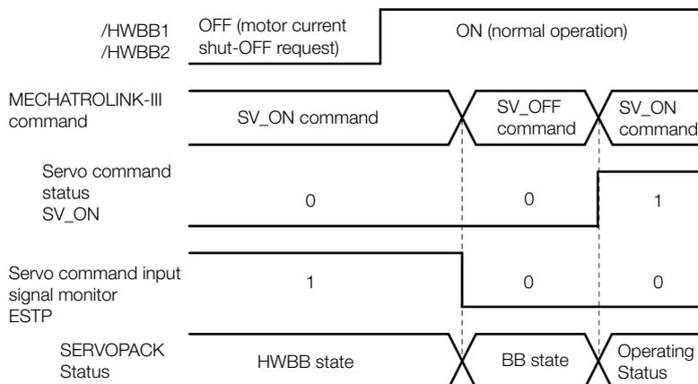
Note: If the SERVOPACK is placed in the BB state while the main circuit power supply is OFF, the HWBB state will be maintained until the SV\_OFF (Servo OFF: 32h) command is received.
