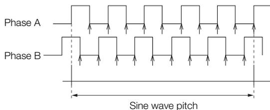
“↑” indicates the edge positions. In this example, the set value is 20 and therefore the number of edges is 20.
