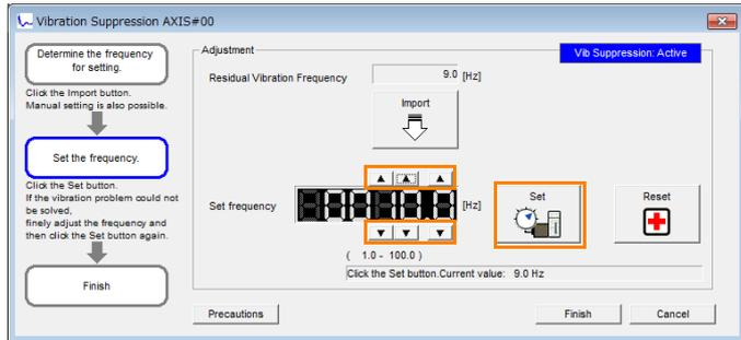
Click the **Reset Button** during adjustment to restore the setting to its original value. The status from before when adjustment was started will be restored.
