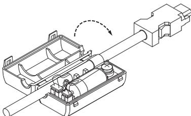
5. Turn OFF the power supply to the SERVOPACK to clear the A.830 alarm (Absolute Encoder Battery Error).
