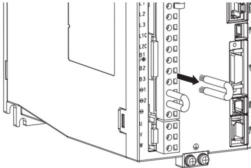
2. Connect the External Regenerative Resistor between the B1/⊕ and B2 terminals.
