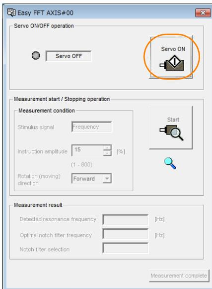
5. Select the instruction (reference) amplitude and the rotation direction in the **Measurement condition Area**, and then click the **Start Button**.
