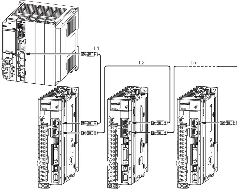
Note: The length of the cable between stations (L1, L2, ... Ln) must be 50 m or less.
