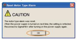
6. Turn the power supply to the SERVOPACK OFF and ON again.
