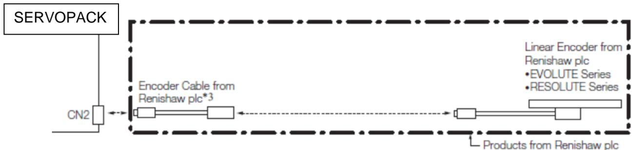
The table below gives the part numbers for varying lengths of the encoder cable to be used that can be purchased from Renishaw.
