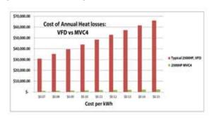
\*Heat loss calculations assume 4400 hour year, 96% operating efficiency for VFD system (including transformers, harmonic filter, fuses and cooling fans).
