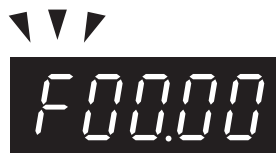
Figure 5.46 Ready for Setting Speed Reference
