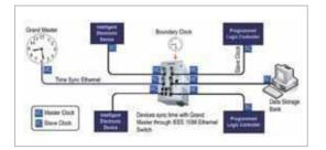
a high level of synchronization within an industrial motion-control environment with a minimum use of network and computing resources. The protocol helps for sequencing event measurements, scheduling outputs, synchronizing actuation, time-stamping, coordinating event records, etc.
