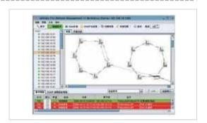
events are updated to the NMS to help users easily maintain the network system. Like as the Korenix NMS, not only supports topology discovery, it also delivers group IP assignment, firmware upgrade, configuration files backup / restore ,SNMP MIB Browser /compile, MSR<sup>TM</sup> group management and also allows user to export topology map to drawing file-JPEG, BMP, PNG or PDF for other application.
