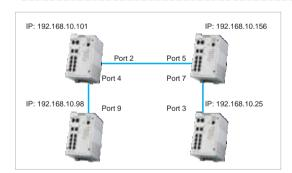
JetNet 5310G supports topology discovery or LLDP (IEEE 802.1AB Link Layer Discovery Protocol) function that can help users to discover multi-vendor's network devices on the same segment by an NMS system which supports LLDP function. With LLDP function, NMS can easily maintain the topology map, display port ID, port description, system description, VLAN ID and so on. Once a link failure happens, the topology changed
