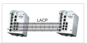
technology. Now, there is no recovery time when failures occur. The JetNet 5010G provides a simple and easy way to aggregate port bandwidth into Rapid Super Ring.
