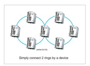
directions. In addition to extensibility, MultiRing<sup>TM</sup> has great diversity of various ring technologies. With MultiRing<sup>TM</sup> enabled, a device can connect RSR<sup>TM</sup> rings, TrunkRing<sup>TM</sup> and a ring of Super Ring together. Which provides extensibility to new technologies while keeping the great backward compatibility.
