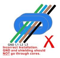
Below is example of multi-conductor cables per phase.
